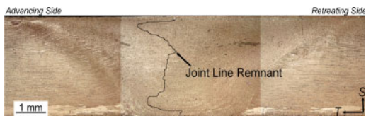
6 Light optical micrograph of weld with JLR: JLR line redrawn artificially to highlight its morphology
