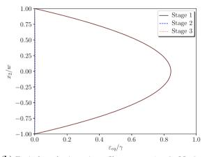
(b) Equivalent plastic strain profiles at stages 1 to 3 of fig.9a, obtained using the proposed model
