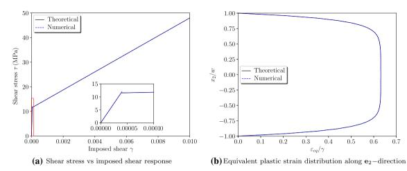
Fig. 5 Simple shear results obtained using the present model
