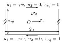
Fig. 2 2D strip subjected to simple shear loading and vanishing plastic stain on the top and bottom edges
