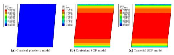
Fig. 10 Distribution of cumulative plastic strain within the studied plate, obtained using imposed tensile strain  $\varepsilon = 2 \gamma = 0.02$ and l/w = 0.4
